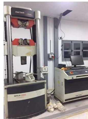
Fig.7: Capacity of Ibertest 1000KN
